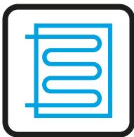
Built with seamless copper tubes and headers, mechanically expanded into corrugated aluminium fin material for a permanent primary to secondary surface bond. Tested at 500 psi, with maximum operating limits at 300 psi.
