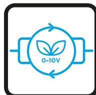
EC motors allow the centrifugal fan to operate at optimum airflow performance, energy efficiency and quiet operation. EC motors include driven control PCB, constant torque, permanent magnet and 3 speeds pre-set or modulating with a 0-10 VDC signal for precise air balancing control.
